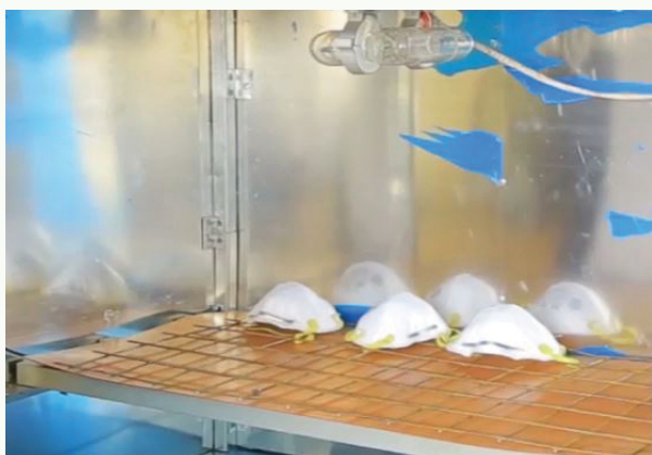
The outside and interior of the Low-cost decontamination equipment for N95 and cloth masks
